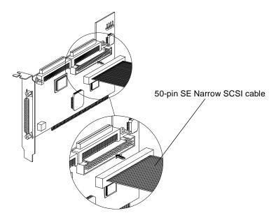
Figure 1-9. Connecting Ultra/Fast Narrow Devices
